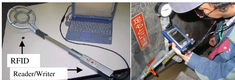
Fig. 4. RFID and reader/writer (left) and an inspector retrieving data from RFID by PDA (right)
